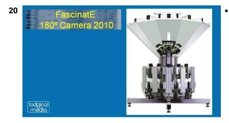
Their next generation used mirrors. The cameras look upwards. Note that the optical centre of *all* the cameras *appears* to be at a point in the very centre of the mirror array. The cameras all view from the same central point. Very clever. Objects can now get close to the camera without influencing the stitching process.
